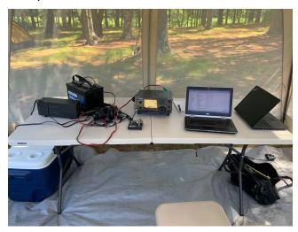
This year, I headed up on Friday morning and set up my station – consisting of an ICOM IC-746Pro and a 40 meter inverted V, situated in one of the screen rooms I bring on Field Day. The 746 ran off battery power, and I turned it down to 5 watts or so in order to conserve battery life. Conditions weren't the best, but on 5 watts rag chewed with people around the country and Europe on 40 meter CW. And I made a few contacts in the contest as well.
